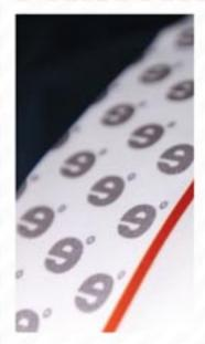
**SUBLIMATION** – The printing service most often delivered by us is sublimation. It is a transfer print technique which consists in transferring graphic design onto sublimation paper. Then, it is transferred onto a polyester material in high temperature environment.
